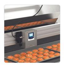
HunterLab inline color measurement systems are versatile and can be seamlessly integrated in existing production line for efficient color quality control of textiles, paper, food, plastics, building materials and coating. Real-time continuous color measurement eliminates the need for time-consuming analysis of samples in the laboratory.
